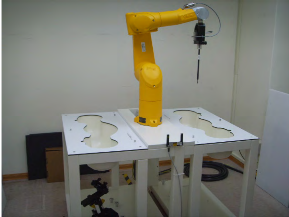
Fig.1 Photograph of the SAR measurement system
