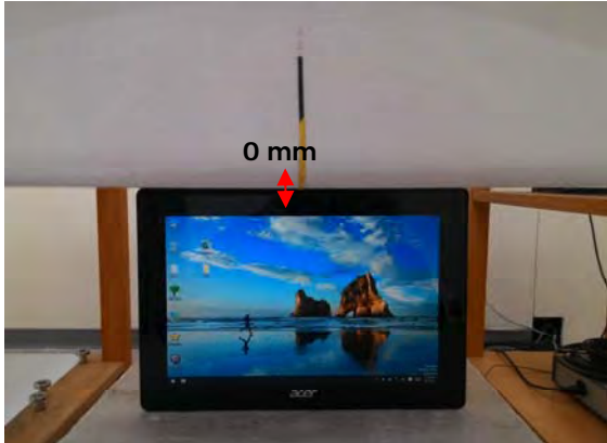
Fig.3 EUT Top side to flat phantom
