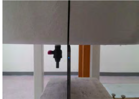
Fig.3 EUT Top side to flat phantom
