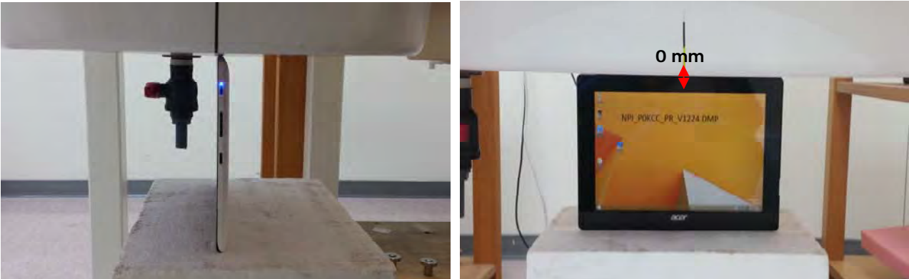
Fig.4 EUT Top side to flat phantom
