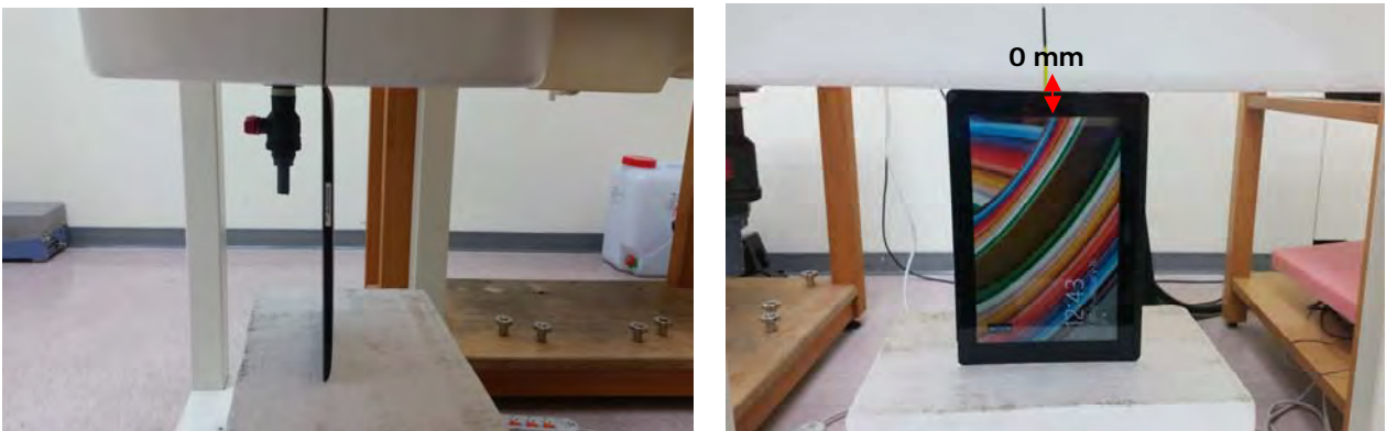
Fig.5 EUT Right side to flat phantom
