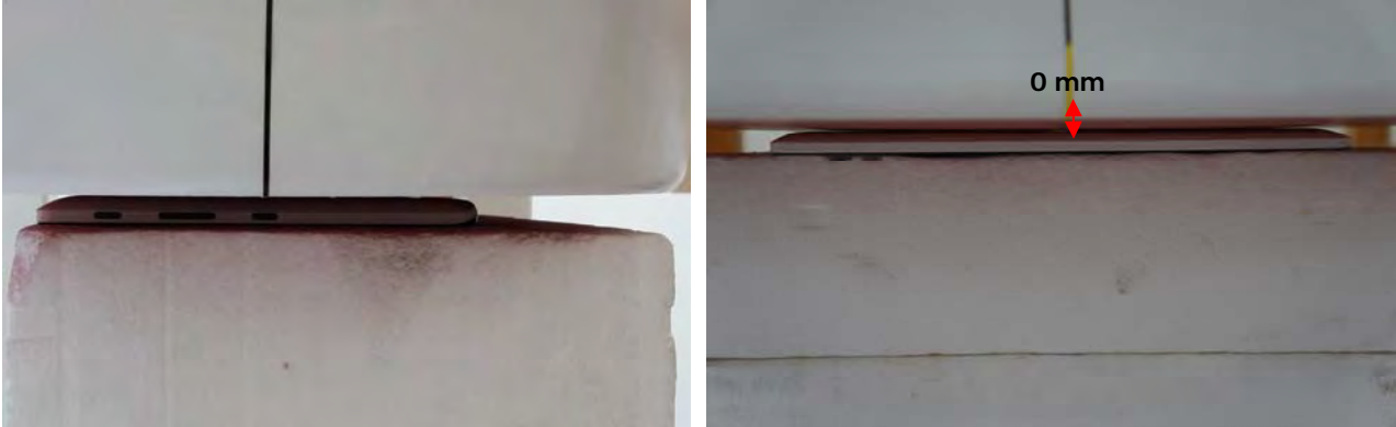
Fig.3 EUT Lap-held mode to flat phantom
