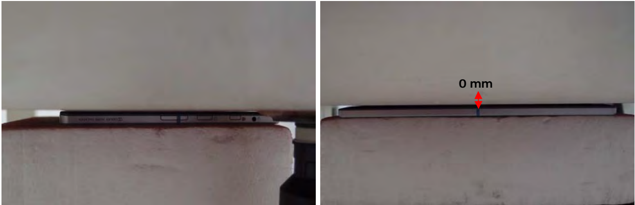
Fig.3 EUT Lap-held mode to flat phantom
