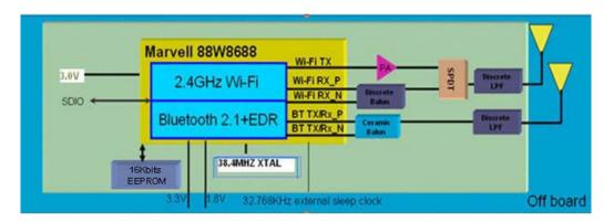
Figure 1 Functional Block Diagram
