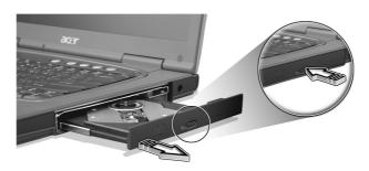
When the power is off, you can eject the drive tray using the emergency eject hole. See page 58.
