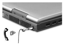
Wrap a computer security lock cable around an immovable object such as a table or locked drawer handle. Insert the lock into the notch and turn the key to secure the lock. Some keyless models are also available.
