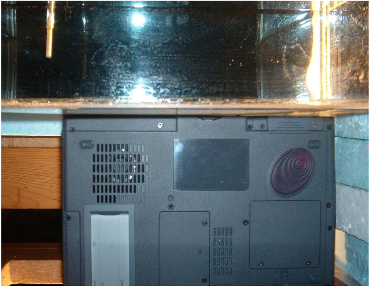
Fig. 4b. Photograph of the Acer TravelMate 660 Notebook Computer with left edge of the PC at 90° pressed against the base of the planar phantom. This is Configuration 2 for SAR testing and represents the case of a bystander in contact (at a distance of 0 cm) with the left edge of the PC.
