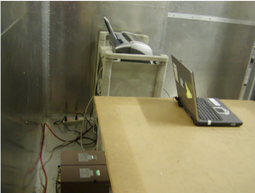
Conducted Emission - Side View, BY27 Antenna
