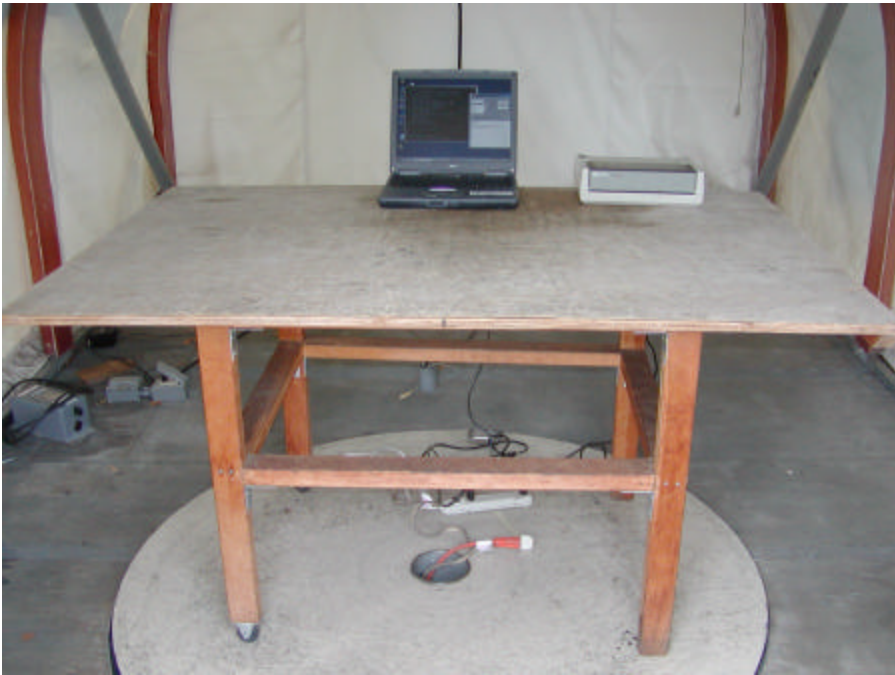
Radiated Emission - Front View, BY27 Antenna
