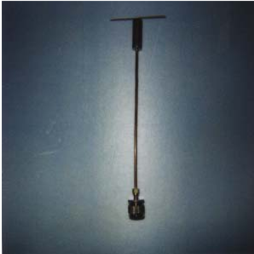
Fig. 15. Photograph of the half-wave dipole at 1900 MHz used for system verification.
