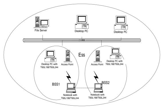
Fig.4 Roaming in an Extended Service Set (ESS)
