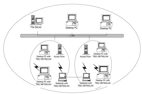
Fig.2 Infrastructure Wireless LAN Configuration
