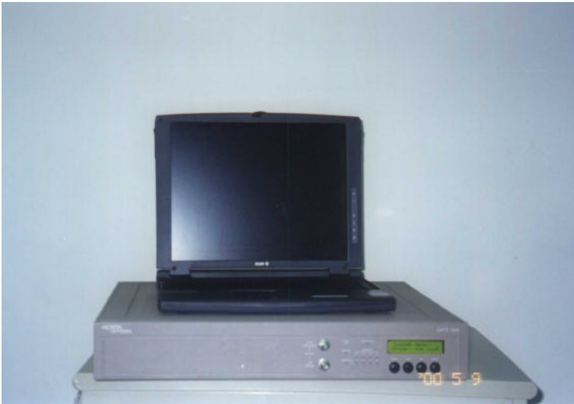
Cable Modem Head End
