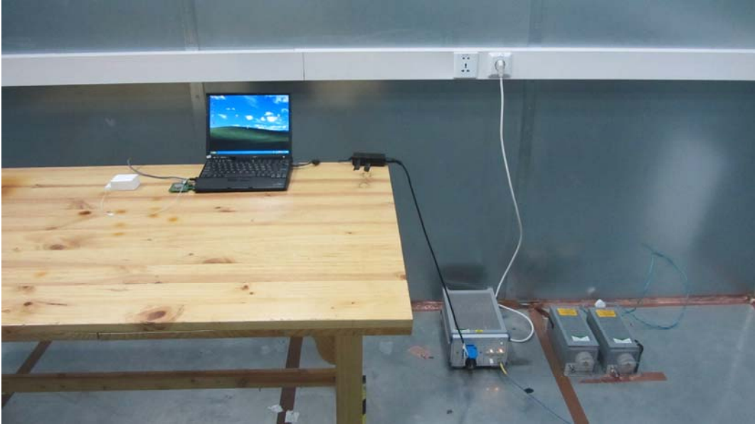
Picture 2 Conducted Emission Test Setup
