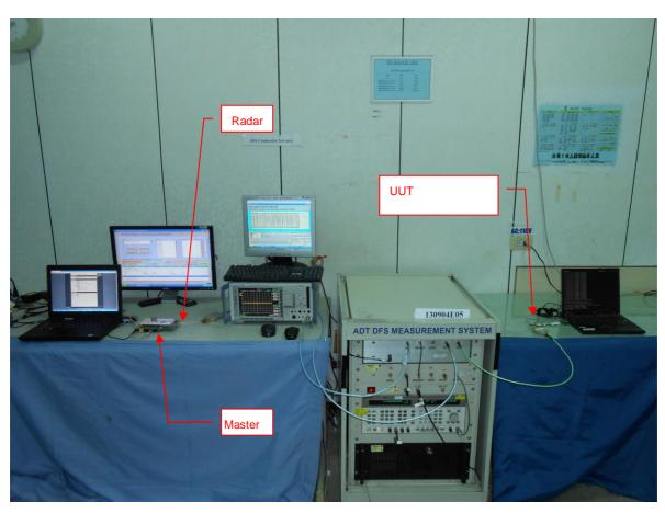
Set UUT as Client without radar detection mode (Radar injected into Master)
