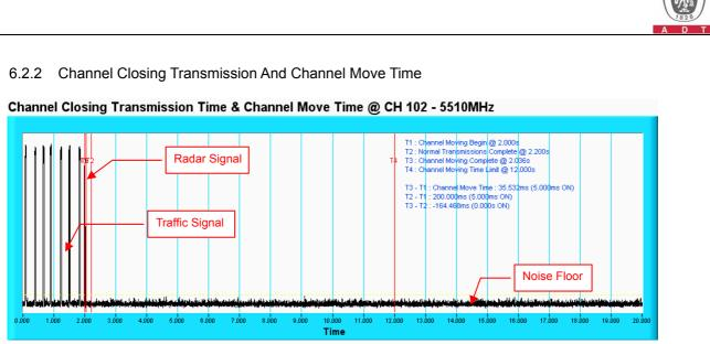
**NOTE:** T1 denotes the start of Channel Move Time upon the end of the last Radar burst. T2 denotes the data transmission time of 200ms from T1. T4 denotes the 10 second from T1 to observe the aggregate duration of transmissions.
