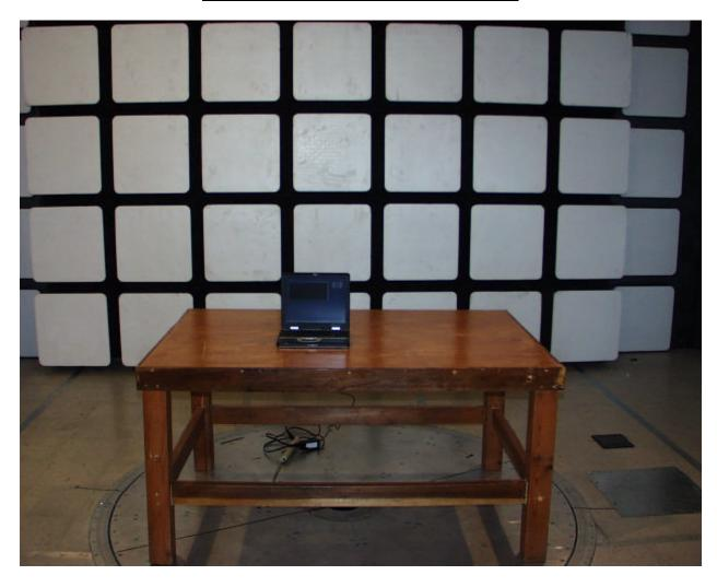
RADIATED RF MEASUREMENT SETUP
