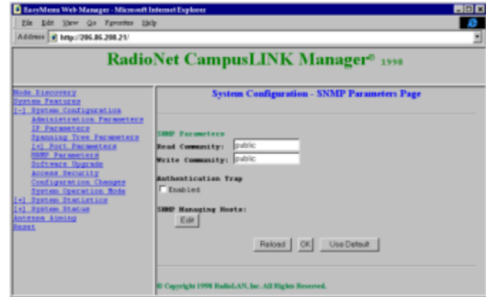
Figure 28: SNMP Parameters Page
