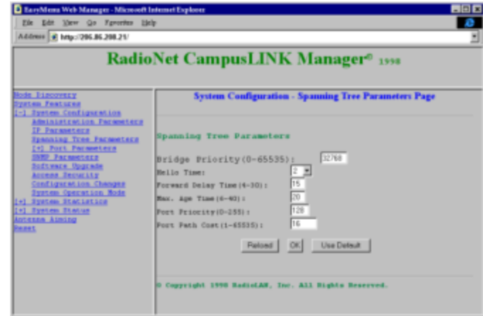
Figure 39: Spanning Tree Parameters Page
