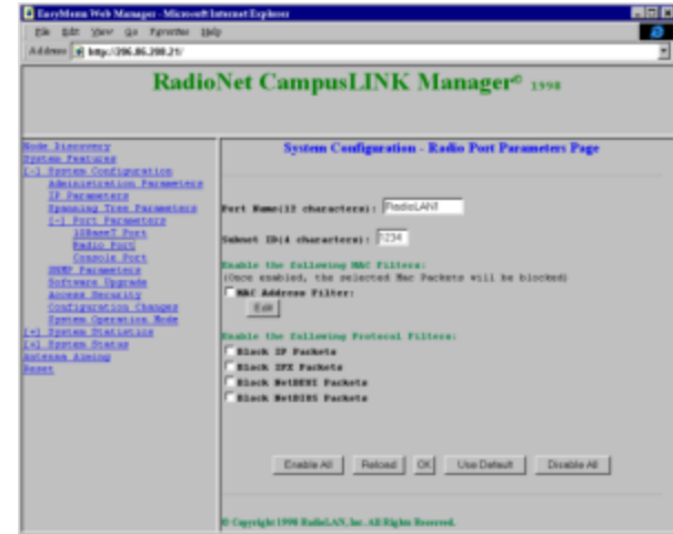
Figure 34: Radio Port Parameters Page
