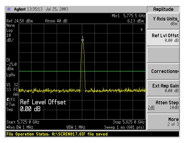
CW output = 6.13 dBm + 10 dB attn + 1 dB CL = 17.13 dBm peak output
