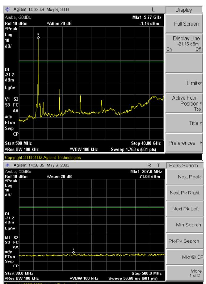
Power Spectral Density Test Requirement: 15.247(d)
