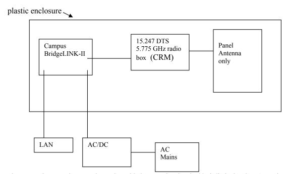
The two products use the same electronics, with the exception that the 387 is limited to the EA panel antenna only. Antenna conducted data is taken at the antenna output of the CRM, and is applicable to both products. The radiated and AC line conducted data taken for one product is applicable to both units. The same schematics, block diagrams, and theory of operation are applicable to both products.
