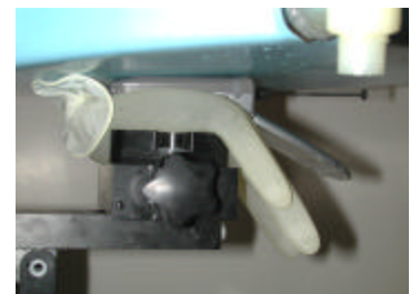
Figure 23. Hand SAR Test Setup
