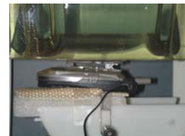
Figure 14.5 Body SAR Test Setup -- w/o Holster --
