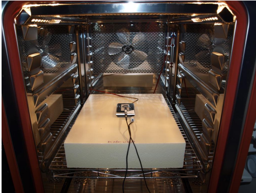
Picture 5: Carrier frequency stability test setup
