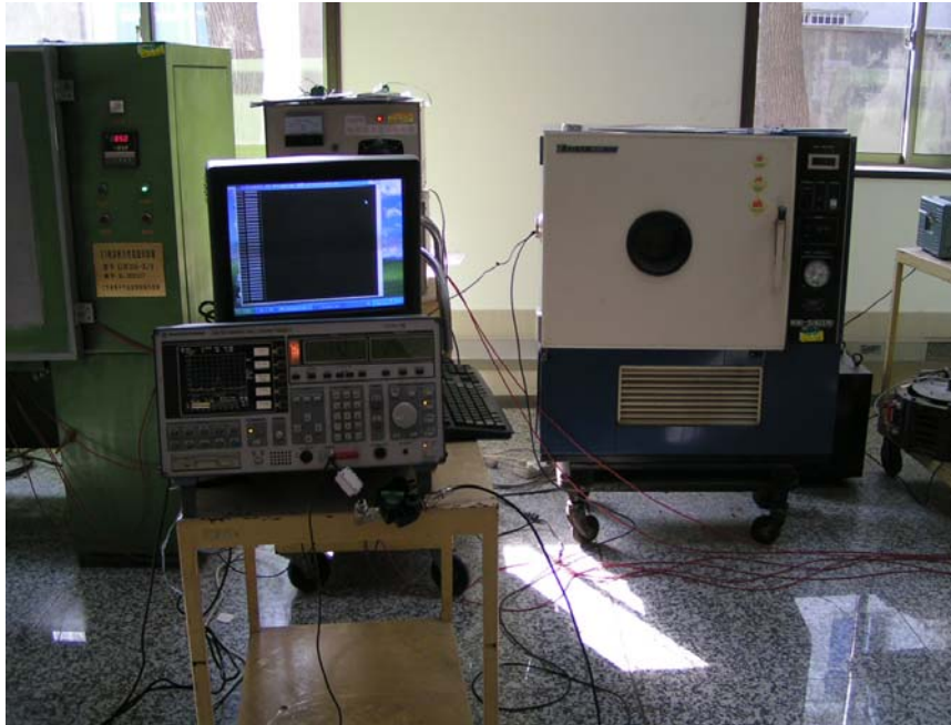
Frequency stability vs. Temperature Test Set-Up
