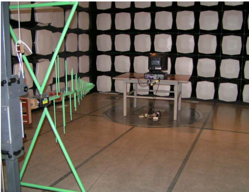
Field Strength Set-up - Rear View
