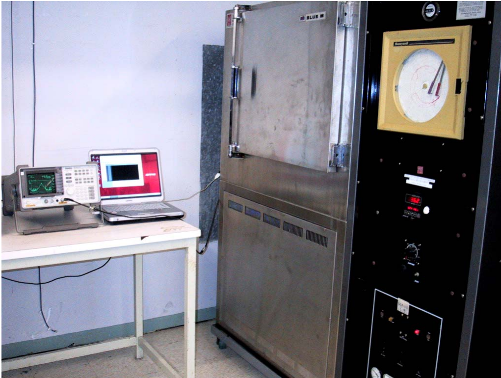
Frequency stability vs. Temperature Test Set-Up
