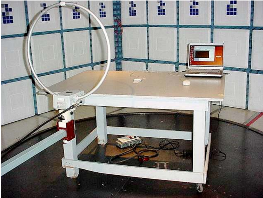
Radiated Emissions at 3m - Front View
