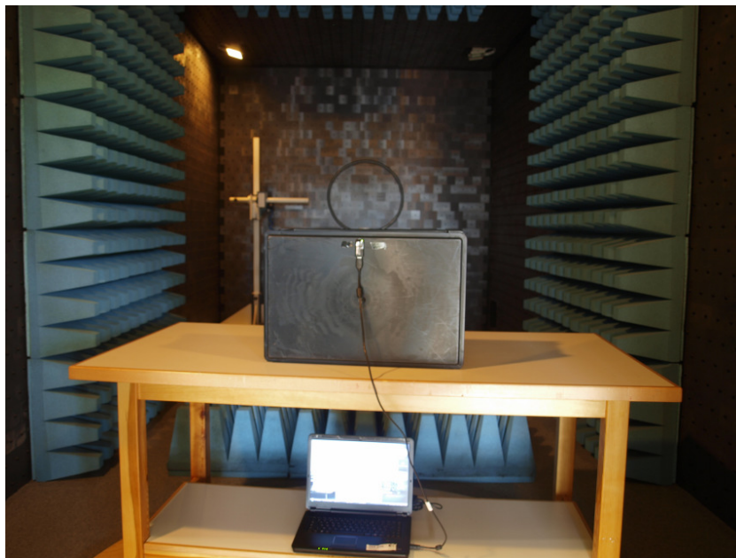
Picture 8: Occupied bandwidth test setup (wide view)
