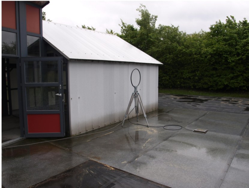
Picture 1: Loop antenna in open site 3m for spectrum mask and radiated emission test
