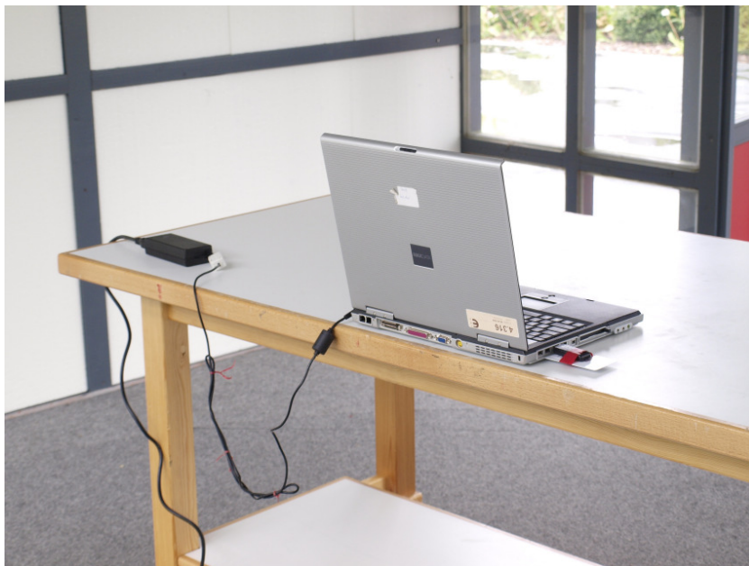
Picture 4: Setup in open site for radiated emission test
