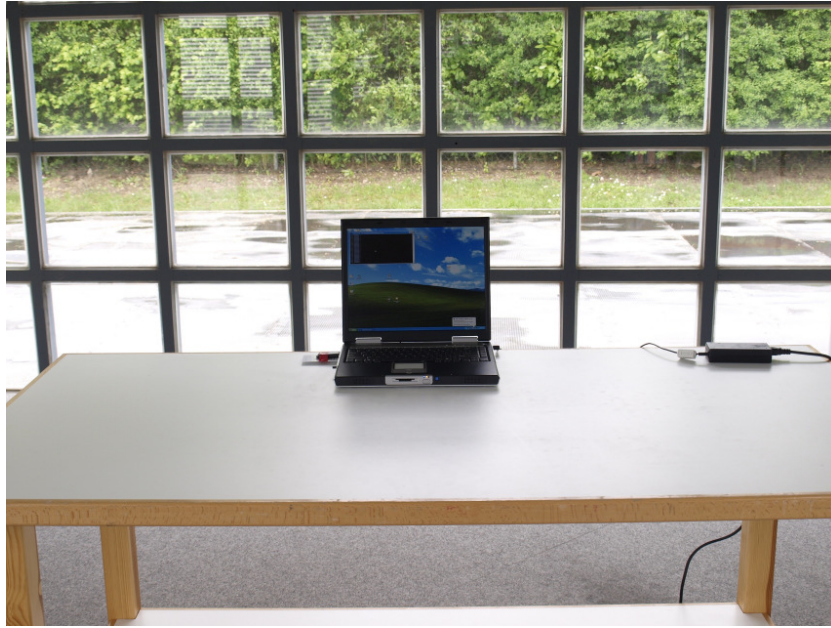
Picture 5: Setup in open site for radiated emission test
