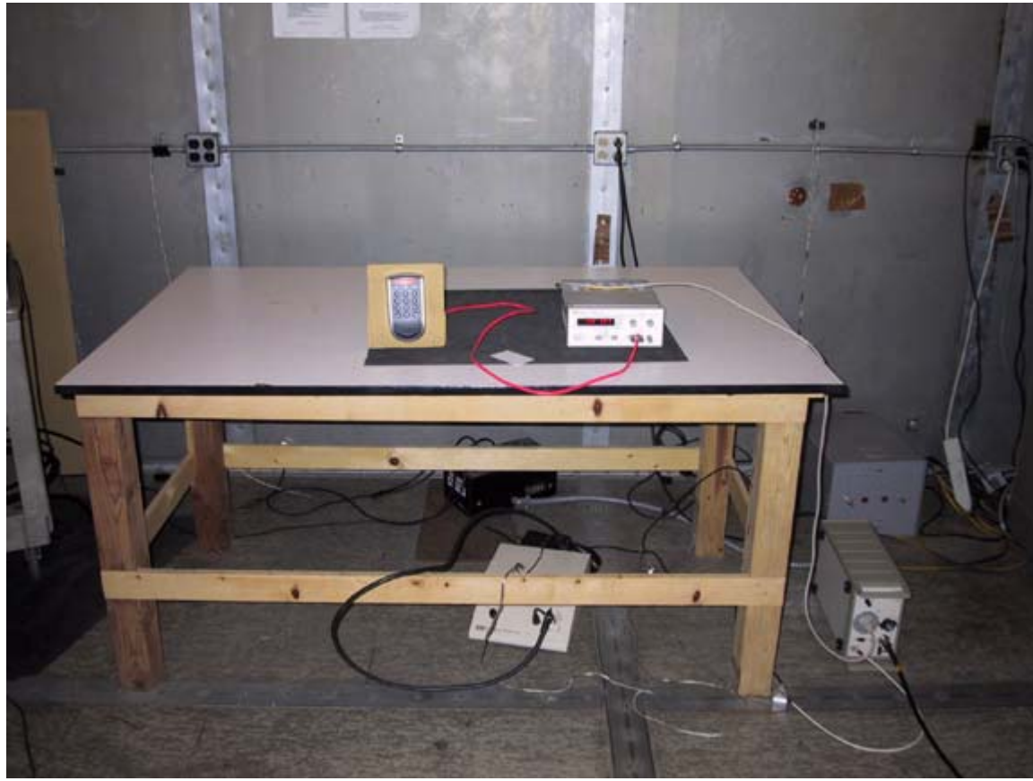
Photograph 3. Conducted Emissions Test Setup
