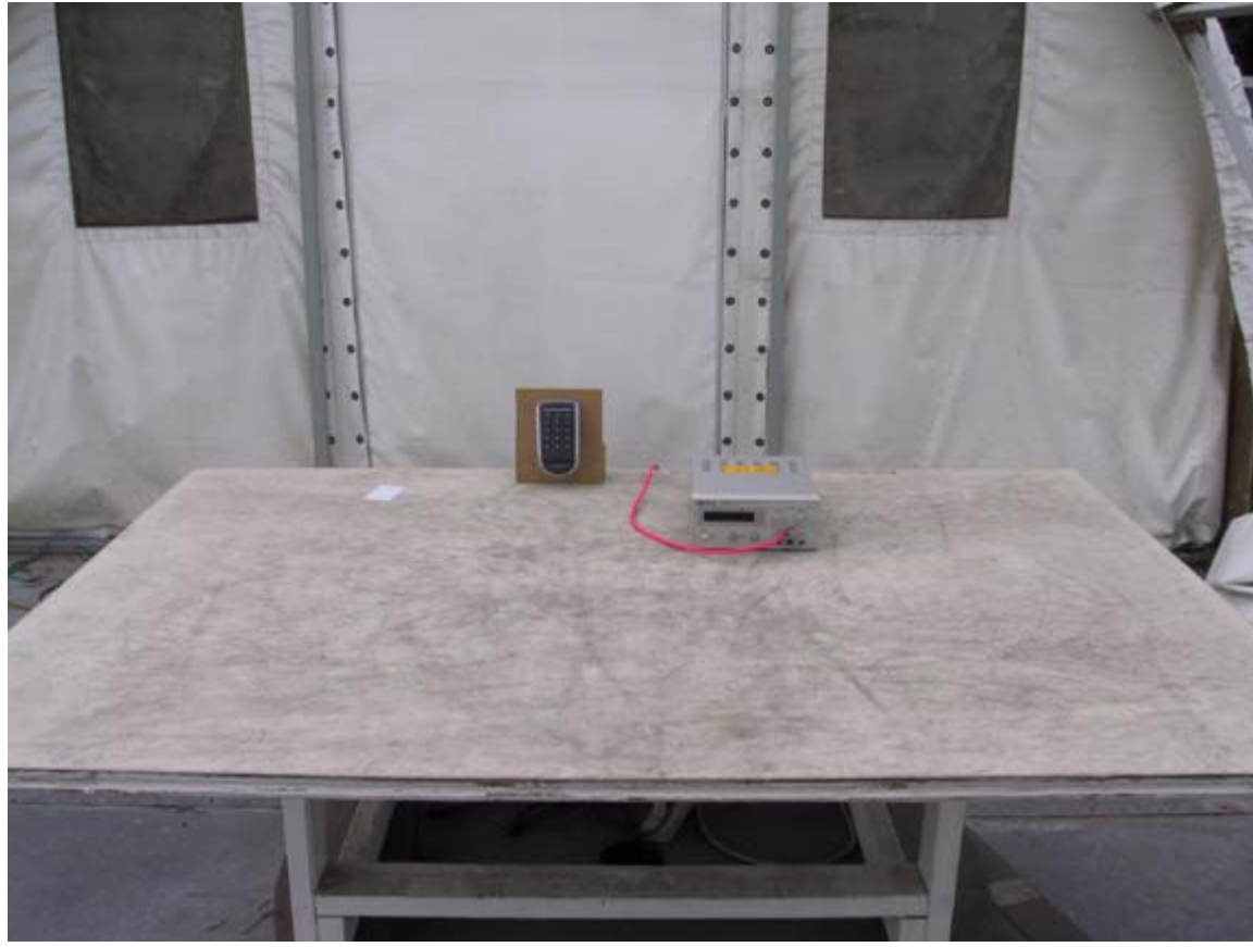
Photograph 1. Radiated Emissions Test Setup (Front View)
