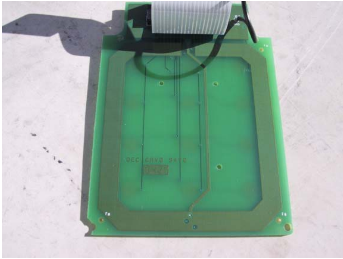
Photograph 1. EUT Internal Photo – Keypad PCB
