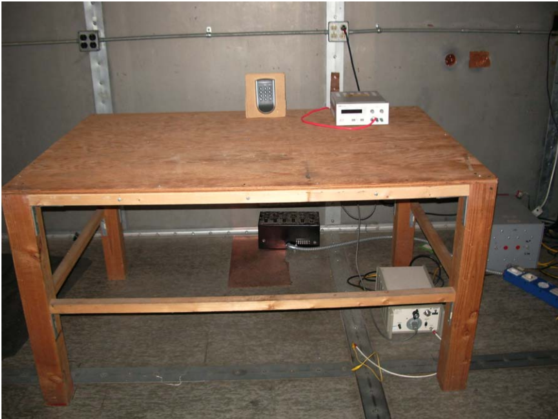
Line Conducted Emissions Setup
