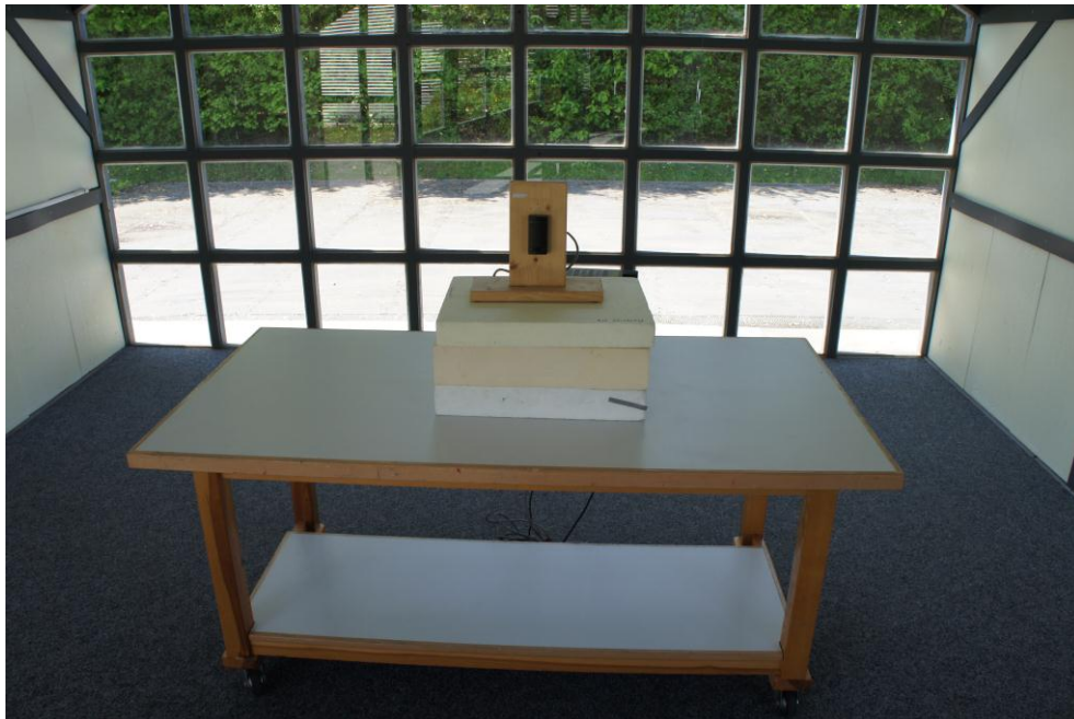
Picture 2: EUT test setup radiated emission test (30MHz to 1000MHz)
