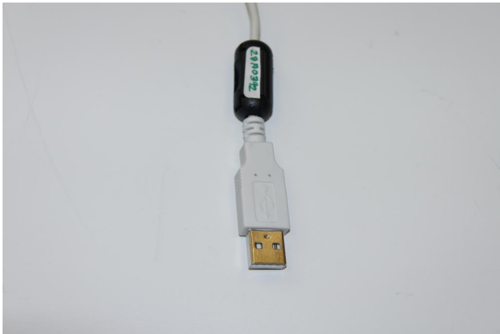
Picture 6: EUT cable with ferrite core
