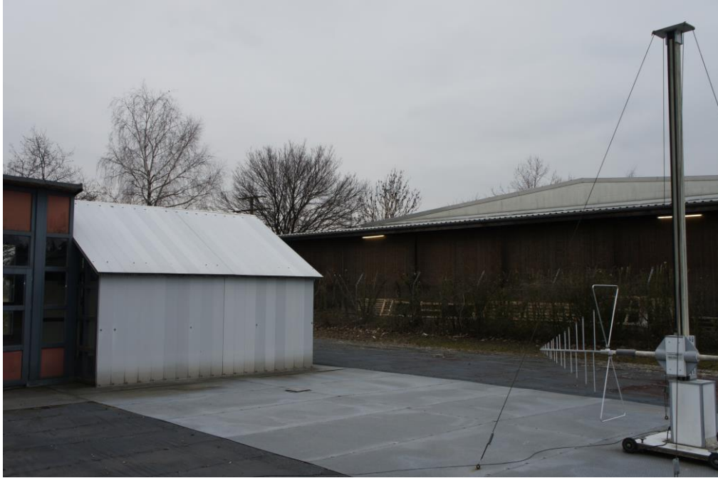
Picture 3: Open site antenna view (30MHz to 1000MHz)
