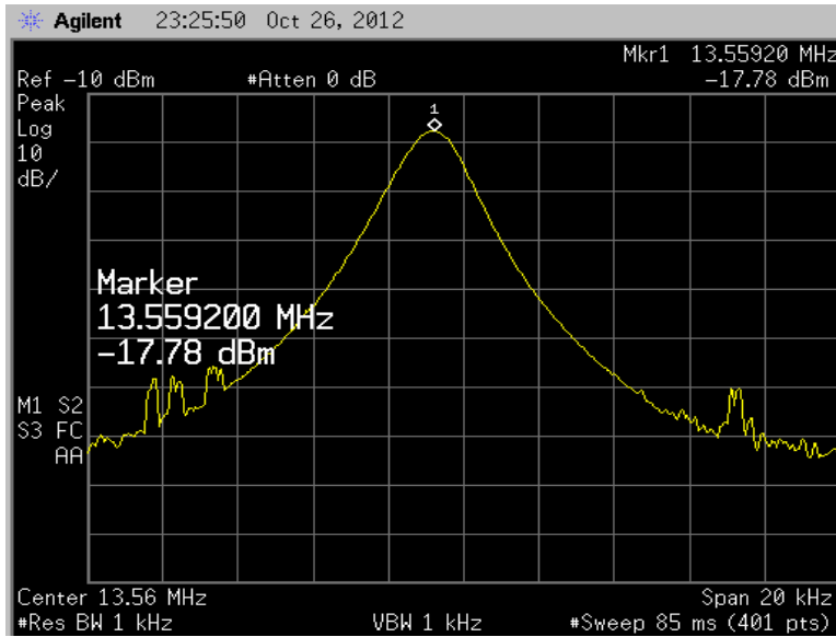
Figure 46: Carrier Frequency at 20°C for 5.75VDC input voltage
