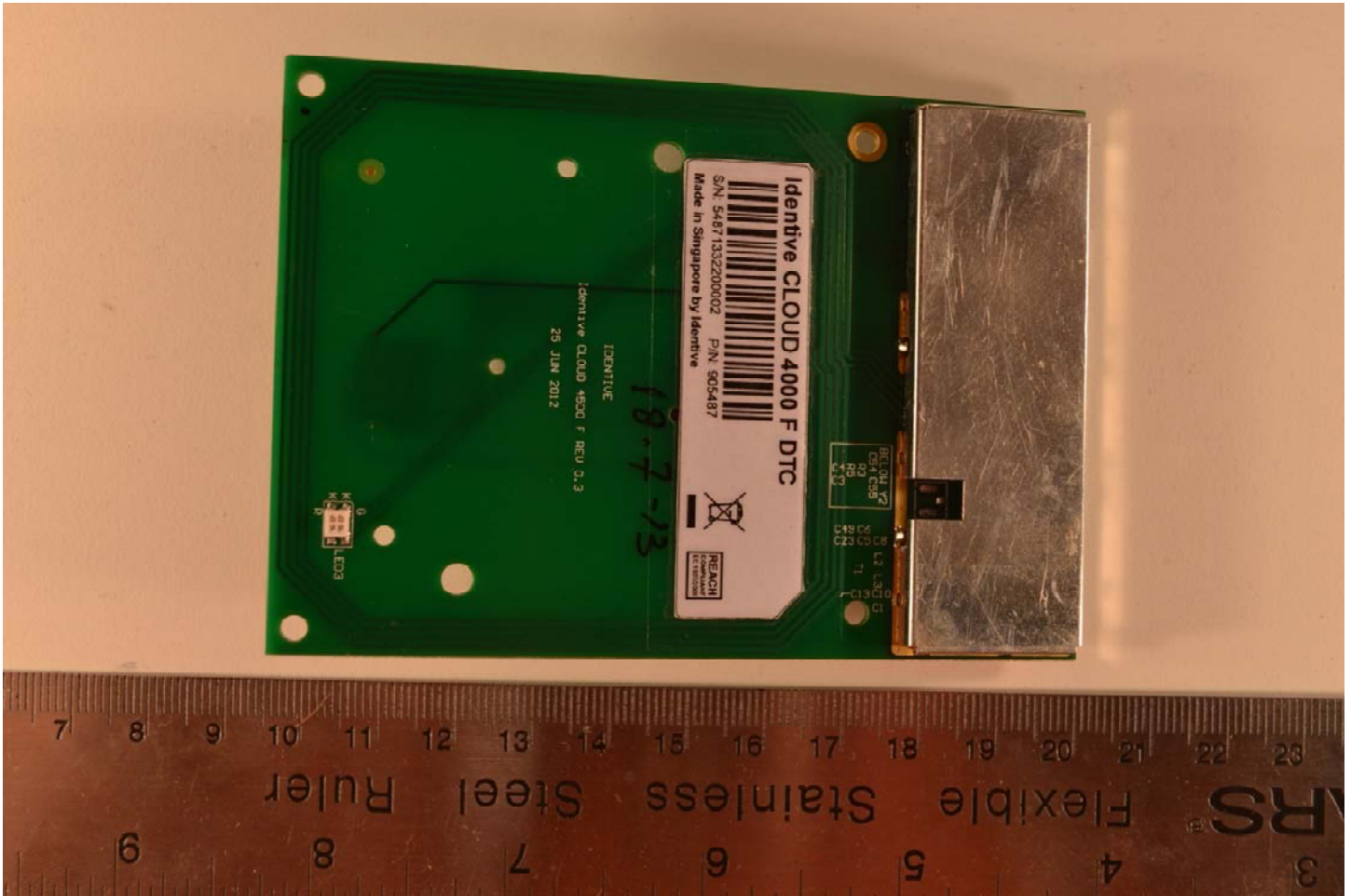
EUT Bottom View [with Radio Shield and printed antenna view]
