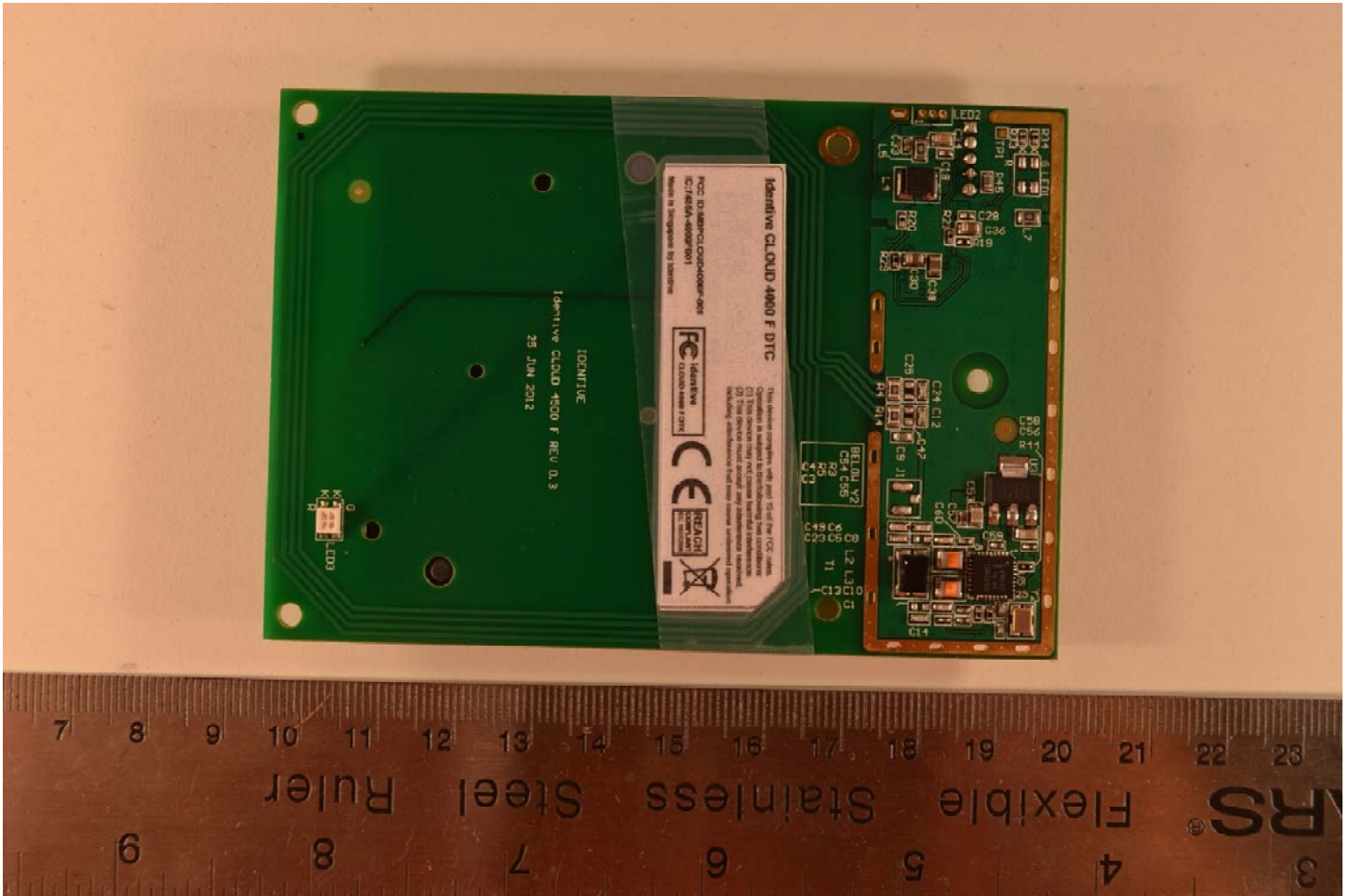
Radio Shield Removed
