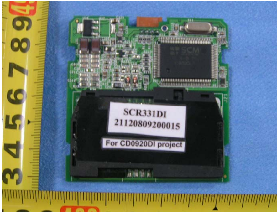
RF Board Front View
