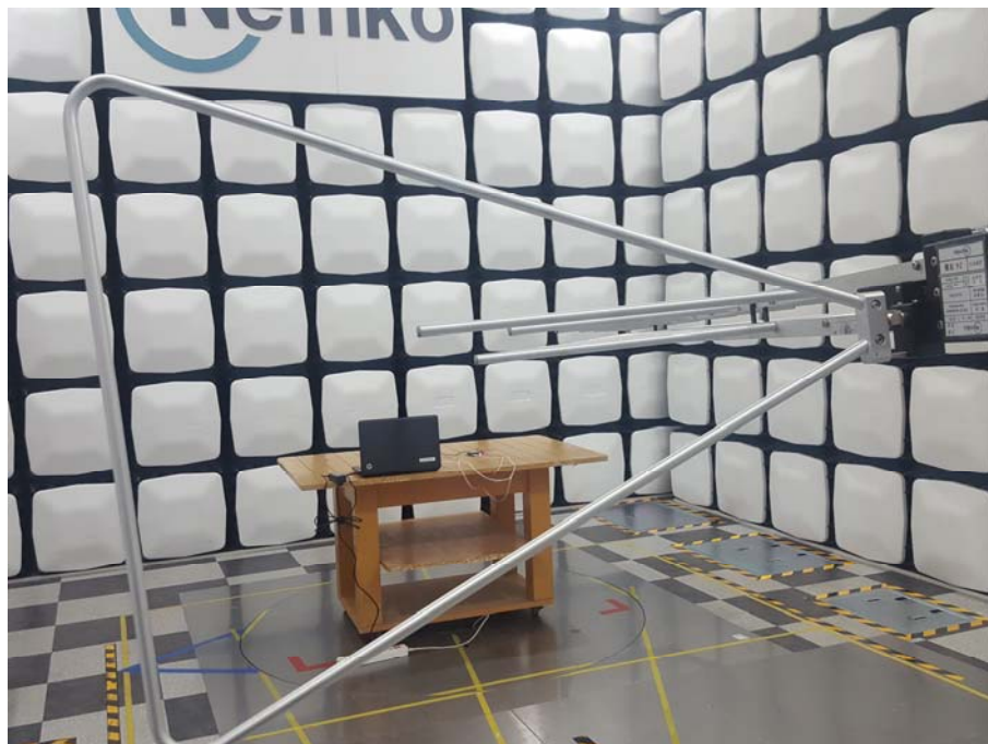
Radiated Test Picture(Rear)_Below 1GHz
