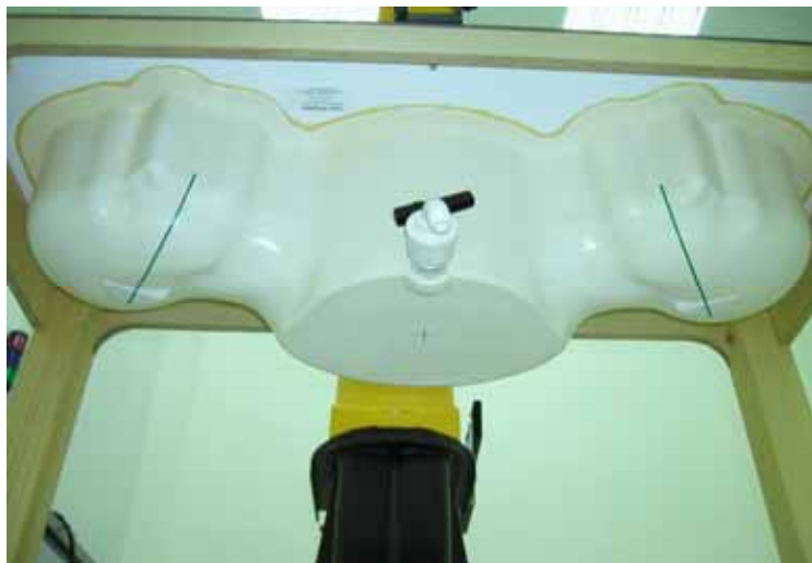
Fig. 5.4 Bottom View of Twin Phantom
