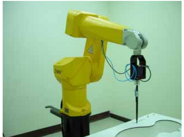
Fig. 5.2 Probe Setup on Robot
