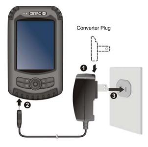
2. The multi-functional indicator glows amber when charging is in progress. Do not disconnect your Pocket PC from AC power until the battery is fully charged. This will take a couple of hours. When charging the battery for the very first time, charge it for at least 8 hours.
