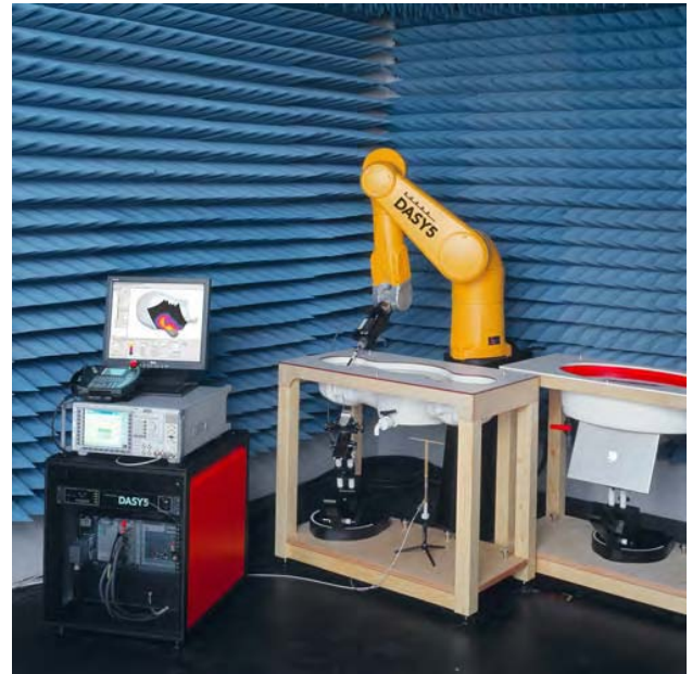
Fig. 5.2 Probe Setup on Robot
