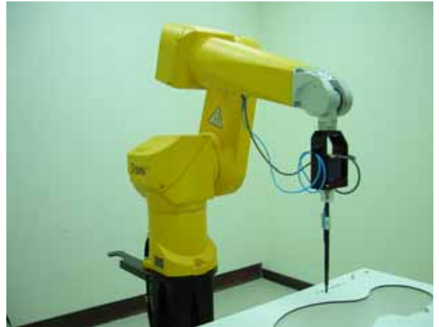
Fig. 5.2 Probe Setup on Robot
