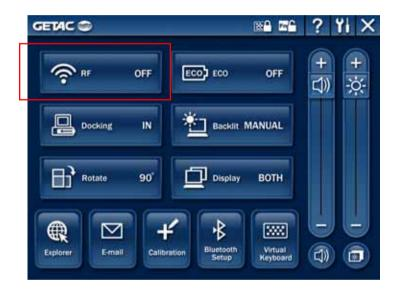
2. Click the RF button to switch the WLAN radio on/off, indicated by the WLAN indicator ( ) glowing in green when on.
