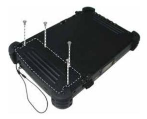
4. Remove the two screws securing the battery pack to the battery compartment (1) and, pull on the ribbon strip to lift the battery pack off the tablet PC (2).
