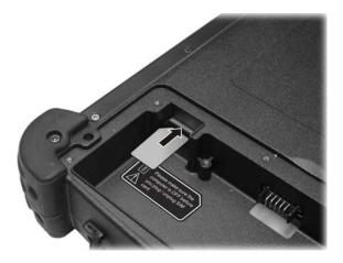
To remove the SIM card, just push in  $(\mathbf{0})$  the SIM card to pop-out  $(\mathbf{2})$  and remove the card.
