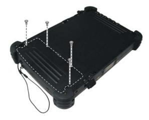
4. Fit the battery pack into place (**1**) and secure with two screws (**2**).
