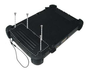
4. Remove the two screws securing the battery pack to the battery compartment (1) and, pull on the ribbon strip to lift the battery pack off the computer (2).
