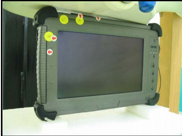
Test Mode 1 ~ 4: The Edge of the EUT face to the phantom with 0mm-separation distance.
