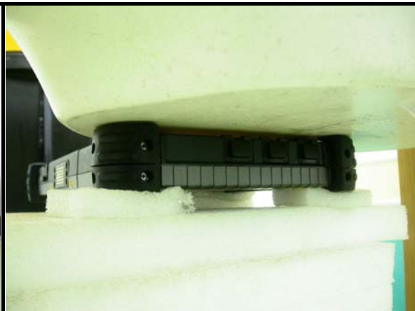
Test Mode 16: The bottom of the EUT face to the phantom with 0mm-separation distance.
