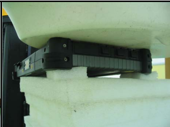
Test Mode 8: The bottom of the EUT face to the phantom with 0mm-separation distance.
