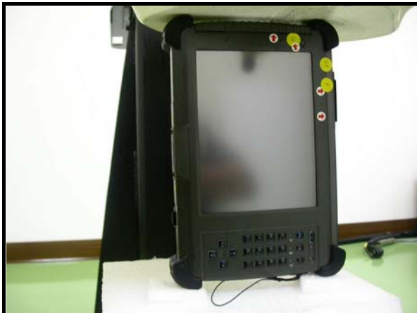
Test Mode 14 ~ 15: The Edge of the EUT face to the phantom with 0mm-separation distance.
