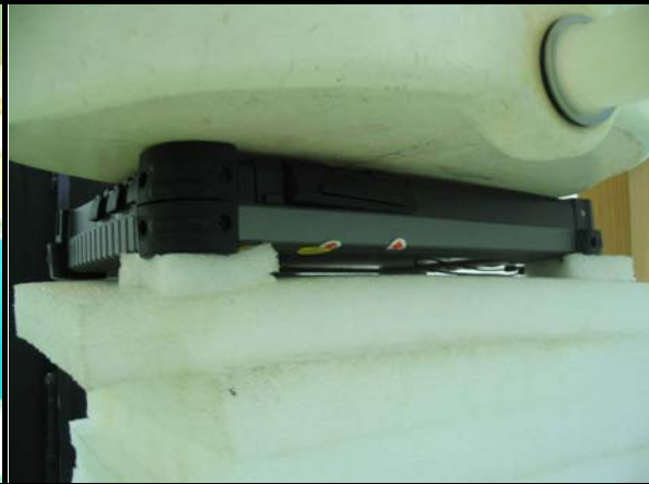
Test Mode 5: The bottom of the EUT face to the phantom with 0mm-separation distance.
