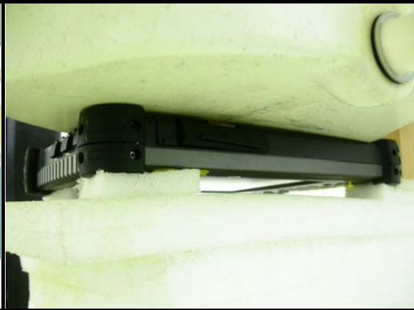
Test Mode 13: The bottom of the EUT face to the phantom with 0mm-separation distance.
