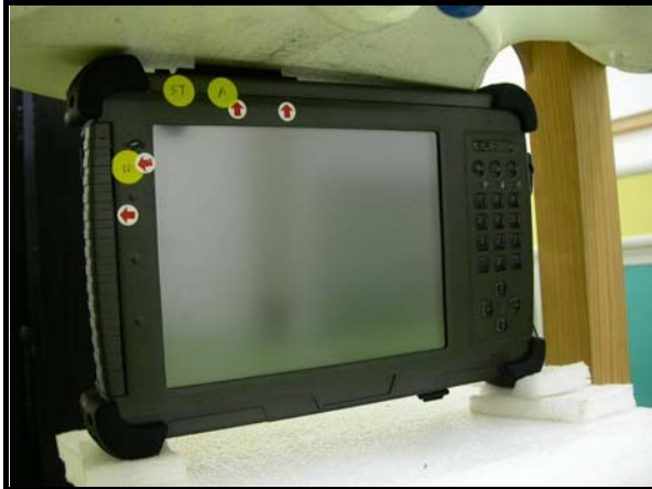
Test Mode 9 ~ 12: The Edge of the EUT face to the phantom with 0mm-separation distance.
