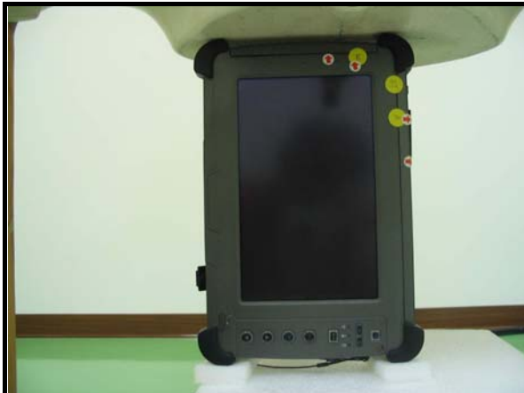
Test Mode 6 ~ 7: The Edge of the EUT face to the phantom with 0mm-separation distance.
