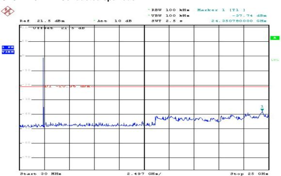
**GFSK 2402MHz Conducted spurious**
