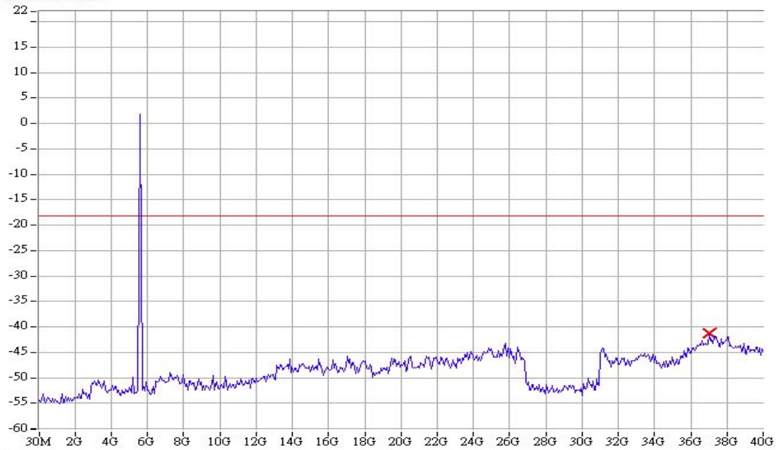
Conducted spurious Chain C 5590MHz HT40
