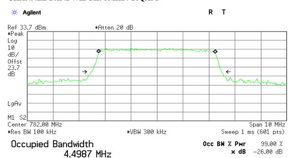
Transmit Freq Error 499.689 Hz x dB Bandwidth 5.031 MHz
