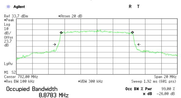
Transmit Freq Error -1.904 kHz x dB Bandwidth 9.481 MHz
