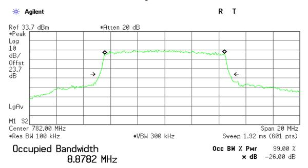
Transmit Freq Error 625.912 Hz x dB Bandwidth 9.621 MHz
