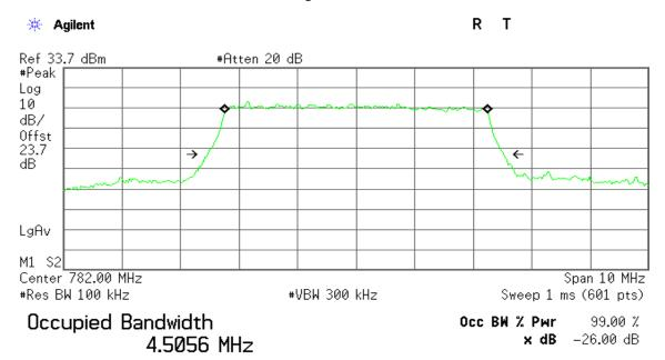
Transmit Freq Error 1.257 kHz x dB Bandwidth 5.066 MHz
