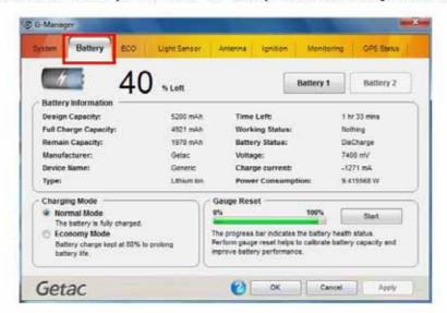
At most two batteries may be supported. Click **Battery 1** or **Battery 2** to view the information of each battery (if your model has a second battery).
