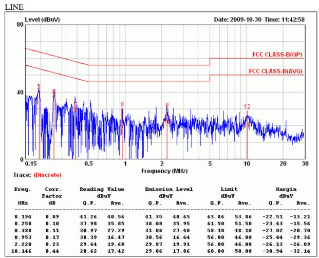
1. Correction Factor = Insertion loss + cable loss
