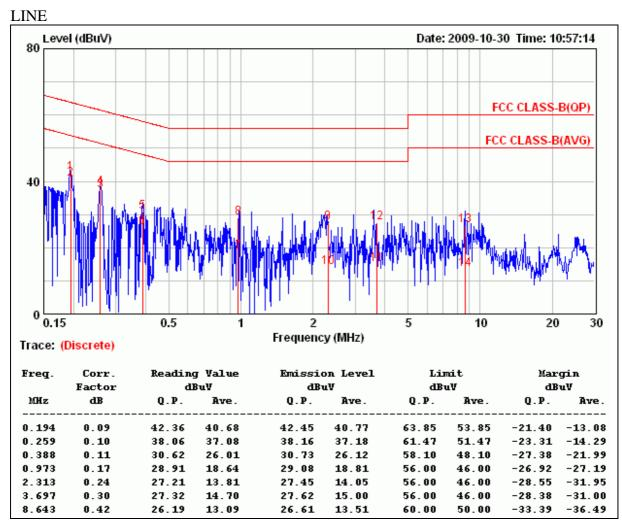
1. Correction Factor = Insertion loss + cable loss
