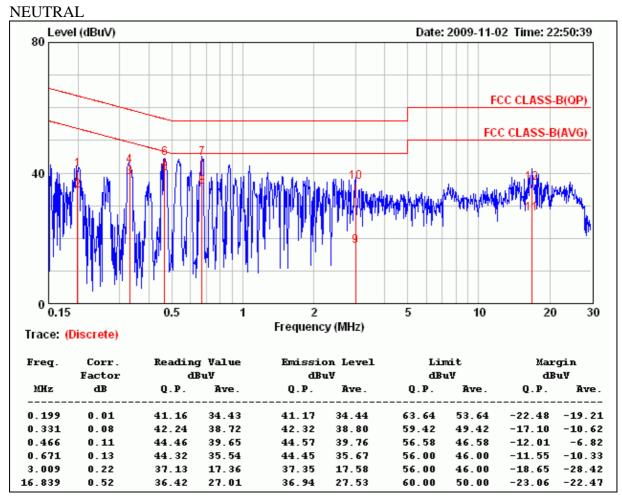
1. Correction Factor = Insertion loss + cable loss
