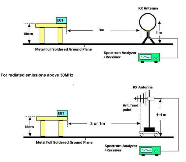
Above 10 GHz shall be extrapolated to the specified distance using an extrapolation factor of 20 dB/decade form 3m to 1m.
